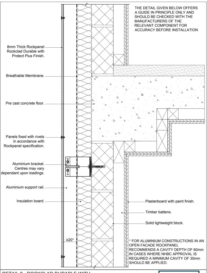
DETAIL 9 - ROCKCLAD DURABLE WITH PROTECT PLUS FINISH VERTICAL SECTION ALUMINIUM SUBSTRUCTURE TO STRUCTURAL CONCRETE & LIGHTWEIGHT BLOCKWORK.
